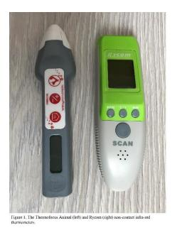
Figure 1. The Thermofocus Animal (left) and Rycom (right) non-contact infrared thermometers.
